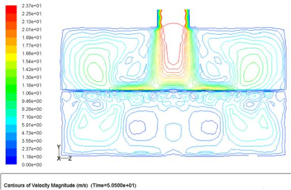
FIGURE 6 Inner streamlines pattern of X=0 section of air jet nozzle
