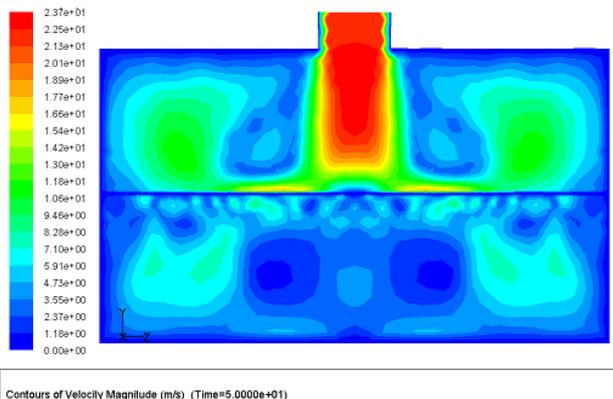
FIGURE 5 Inner flow field of X=0 section of air jet nozzle
