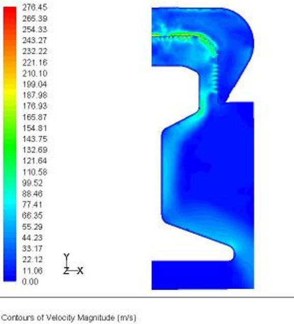
FIGURE 7 The flow field about sections of z=10mm
