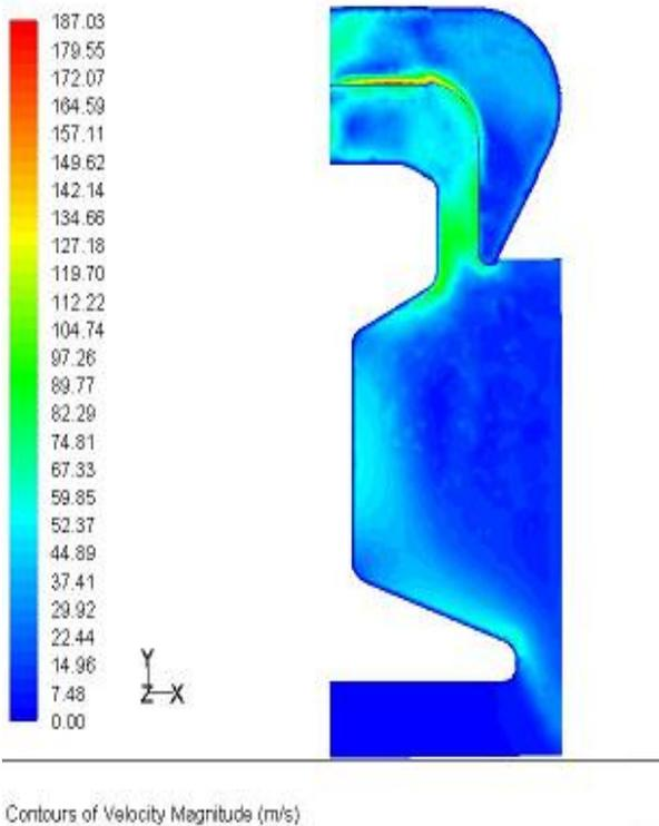
FIGURE 11 The flow field about sections of z=30mm
