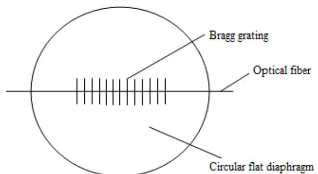
FIGURE 3 Paste position of fiber Bragg grating in the round flat diaphragm
