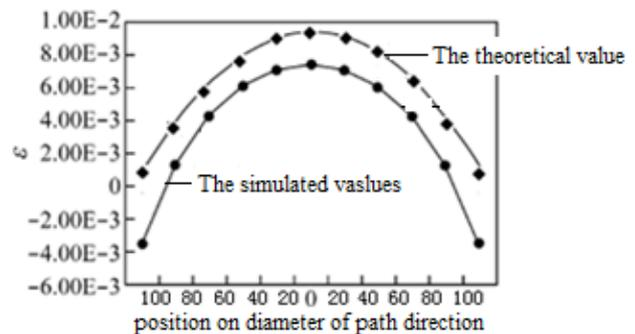
FIGURE 2 Strain of circular flat diaphragm in diameter direction
