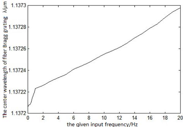
FIGURE 4 Corresponding relations between the given input frequency and the center wavelength about fiber Bragg grating
