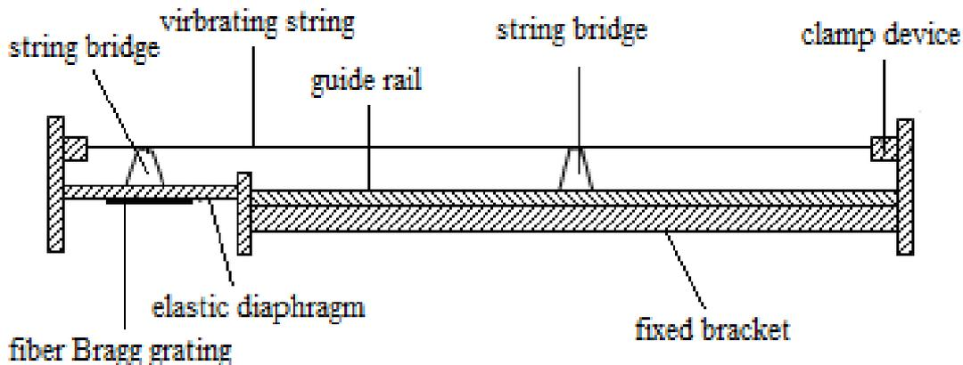
FIGURE 1 The structure of the vibrating wire infrasound sensor based on fiber Bragg grating
