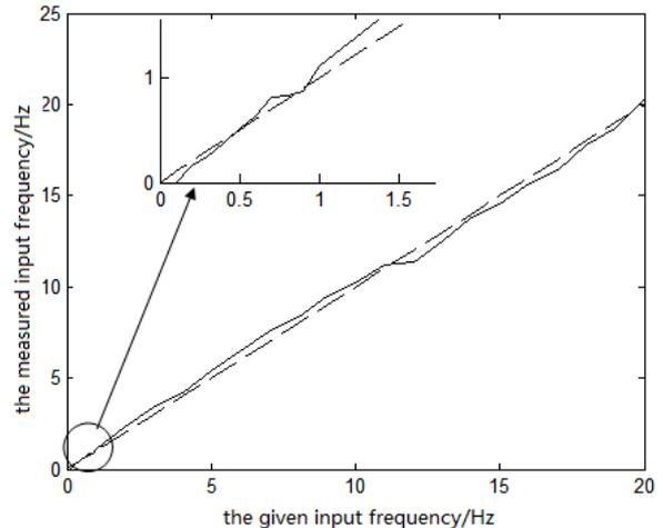
FIGURE 5 The comparison chart between the input frequency (dashed line) and the actual output frequency (solid line)
