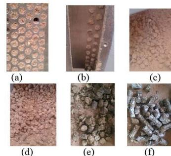
FIGURE 10 The compression experiments of the new biomass pellet forming machine a) Material extrusion condition at the entrance end of forming holes after 10 minute sawdust feed. b) Discharge condition at the outlet end of forming holes after 10 minute sawdust feed. c) Biomass pellet product after 10 minute sawdust feed. d) Biomass pellet product after 20 minute sawdust feed. e) Pellet fuel made by sawdust after 30 minute operation. f) Pellet fuel made by paper scraps after 40 minute operation
