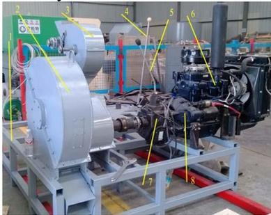
FIGURE 9 The biomass forming system with plunger roller and ring-die at room temperature 1) Frame. 2) Forming mechanism. 3) Drum chipper. 4) Clutch lever. 5) Gearbox lever. 6) Changchai ZN845Q diesel engine. 7) NJ130 Gearbox. 8) Clutch
