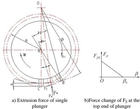
FIGURE 3 The force schematic of the plunger roller
