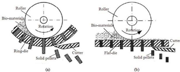
FIGURE 2 The traditional rolling ring-die forming mechanism
