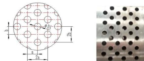
a) Layout of forming holes in the ring-die b) Actual forming holes
