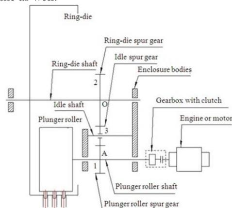
FIGURE 5 The general design of the new biomass pellet forming mechanism
