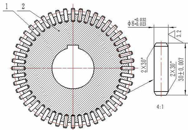
FIGURE 7 The structure schematic of plunger roller. 1) The plunger body 2) The roller body
