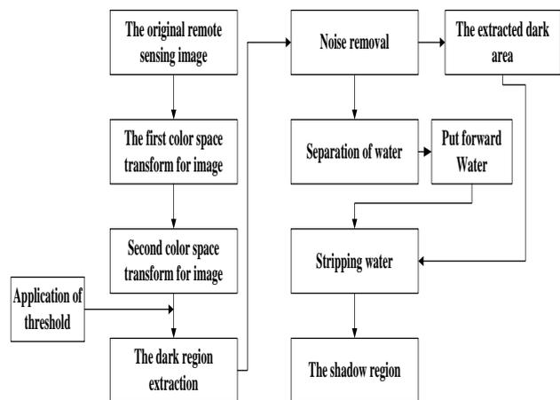
FIGURE 3 Flow chart of shadow detection algorithm
