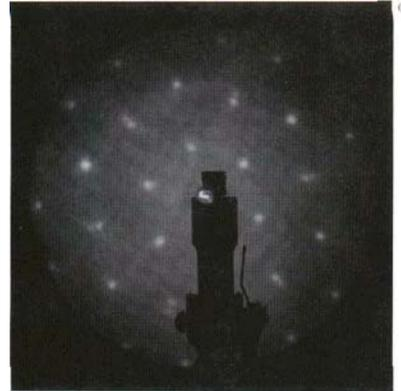
Figure 2. LEED pattern of 50 Å Cu film on  $\alpha$ - $\text{Al}_2\text{O}_3(0001)$  substrate after annealing to 923 K to give Cu(111) particles [7]. The schematic below shows the Cu(111) spots as small, filled dots, and the clean  $\alpha$ - $\text{Al}_2\text{O}_3(0001)$  spots as open circles.
