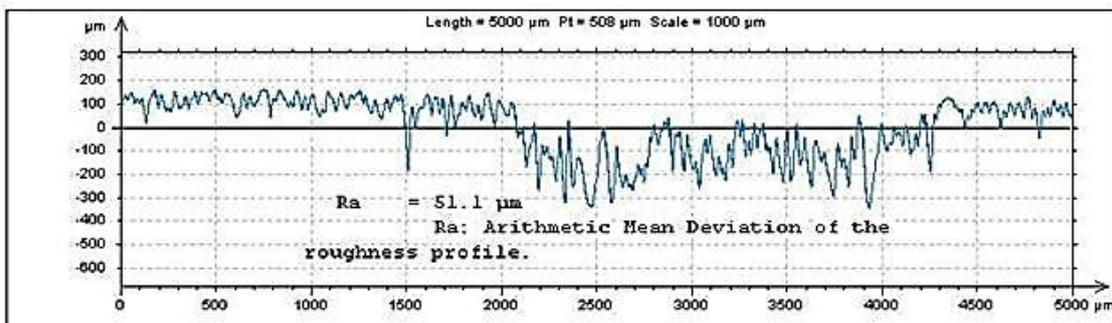
Figure 12. Surface roughness  $R_a$  for test conducted at 150°C
