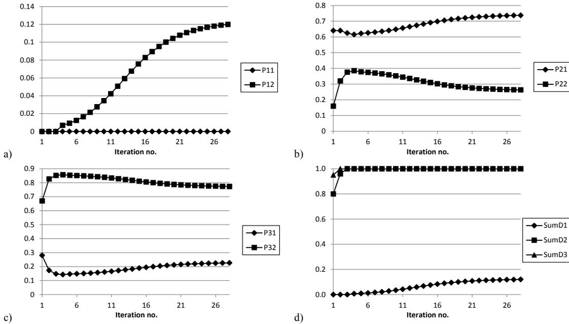
Figure 3. Iterations of the modified adjustment algorithm for the model 2 and the goal  $F_G = [F_0^1, 2 \cdot F_0^2]$ : variation of the repair probabilities in the deterioration states  $D1 \div D3$  (a ÷ c) and sums of repair probabilities in each state (d)
