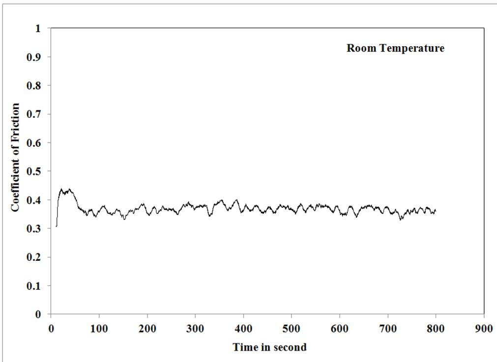
Figure 2. Variation of Coefficient of friction with respect to time at Room temperature
