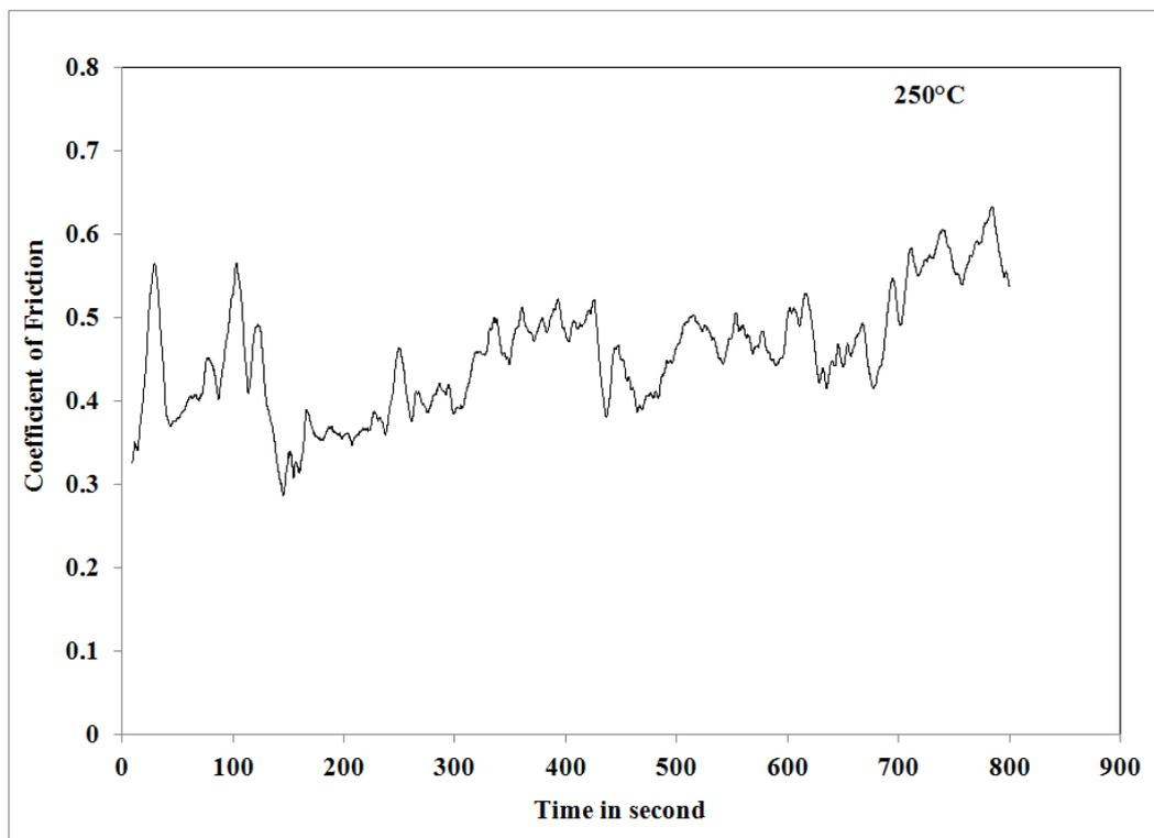
Figure 5. Variation of Coefficient of friction with respect to time at 250°C
