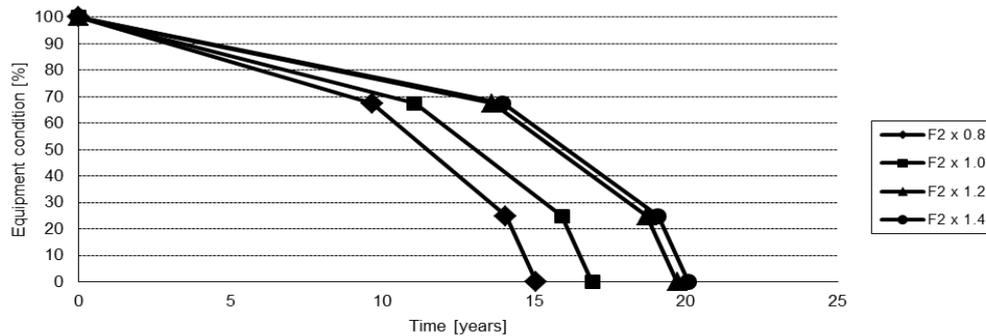
Figure 5. Life curves computed from Markov models adjusted to different frequencies of the major repair
