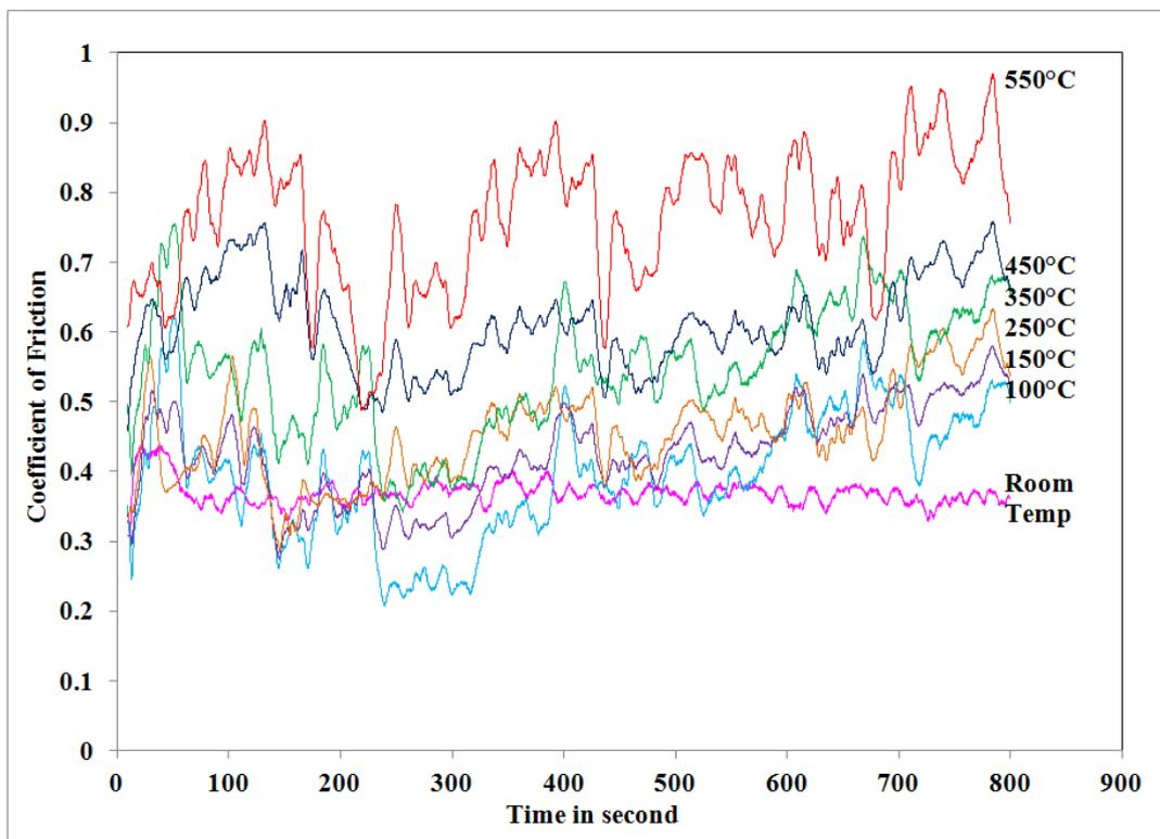
Figure 9. Variation of Coefficient of friction at different temperatures
