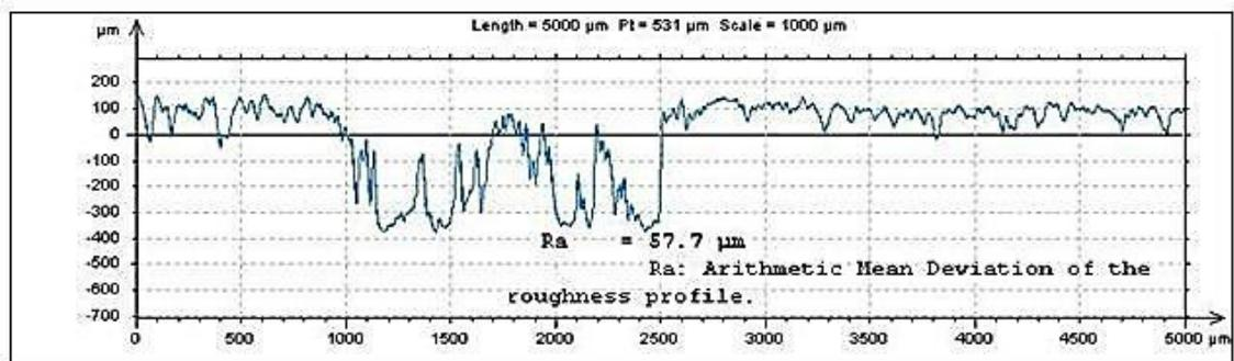
Figure 13. Surface roughness  $R_a$  for test conducted at 250°C
