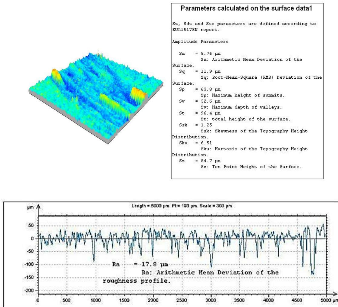
Figure 10. Surface roughness  $R_a$  for test conducted at 25°C
