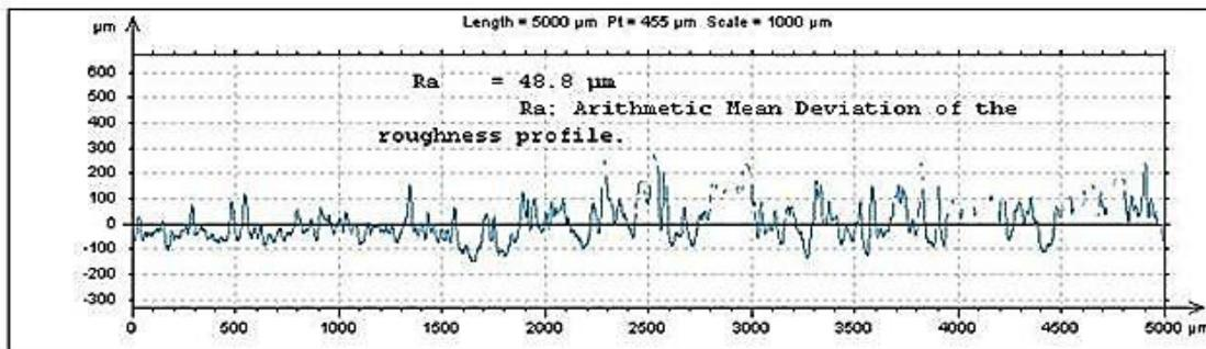
Figure 11. Surface roughness  $R_a$  for test conducted at 100°C
