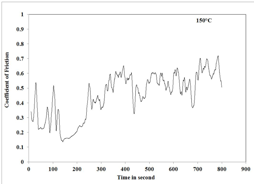
Figure 4. Variation of Coefficient of friction with respect to time at 150°C
