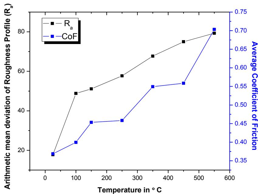
Figure 17. Variation of Surface roughness value ( $R_a$ ) with respect to temperature
