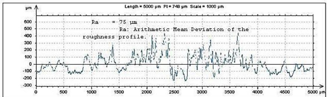
Figure 14. Surface roughness  $R_a$  for test conducted at 350°C
