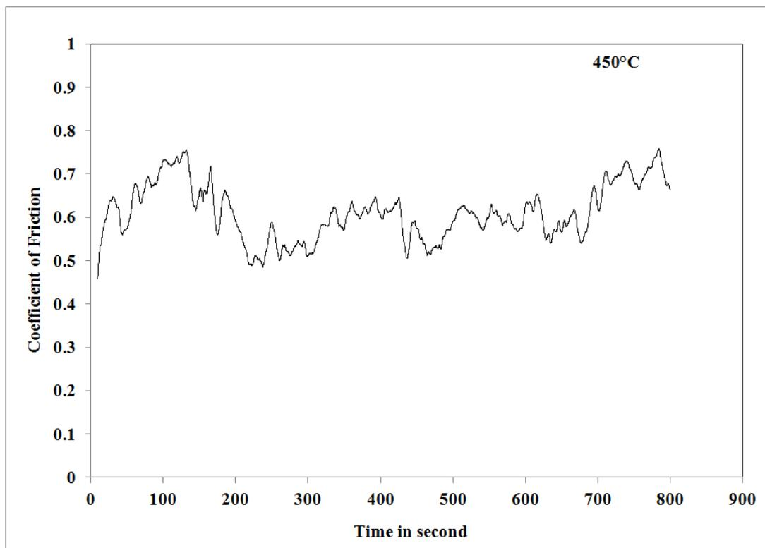
Figure 7. Variation of Coefficient of friction with respect to time at 450°C
