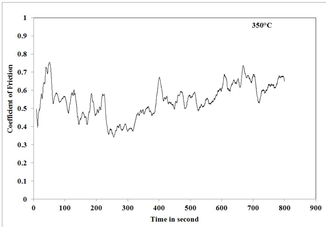
Figure 6. Variation of Coefficient of friction with respect to time at 350°C
