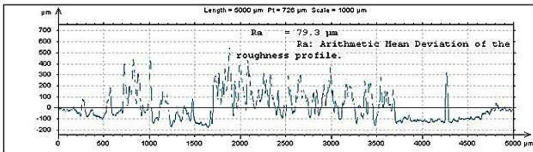
Figure 16. Surface roughness  $R_a$  for test conducted at 550°C
