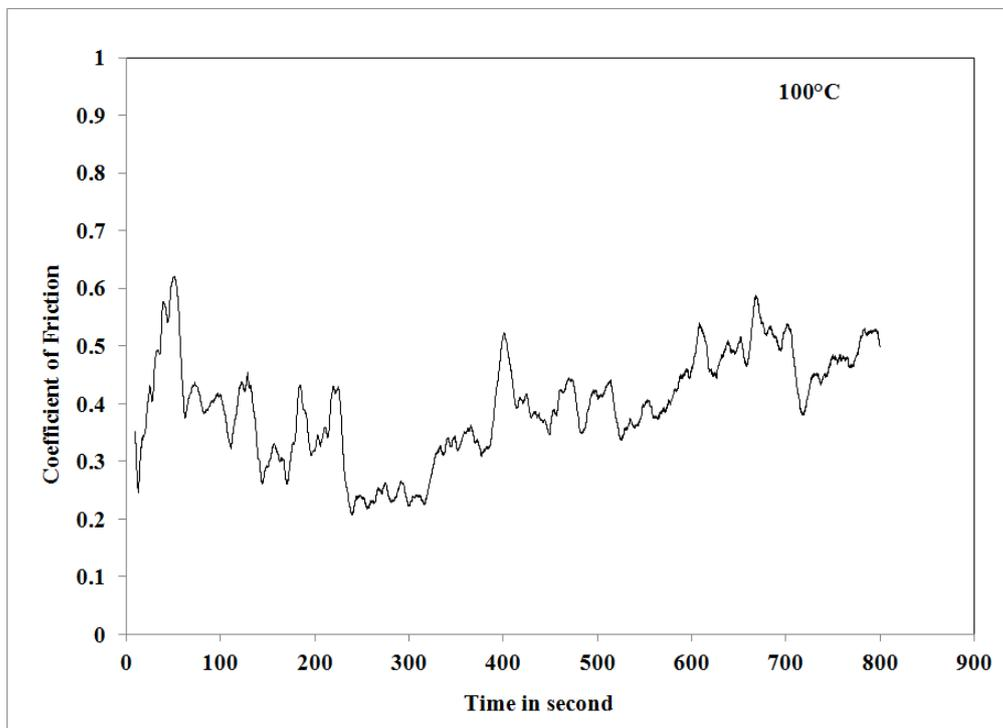
Figure 3. Variation of Coefficient of friction with respect to time at 100°C
