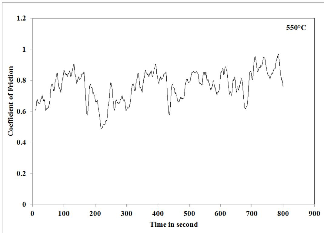
Figure 8. Variation of Coefficient of friction with respect to time at 550°C
