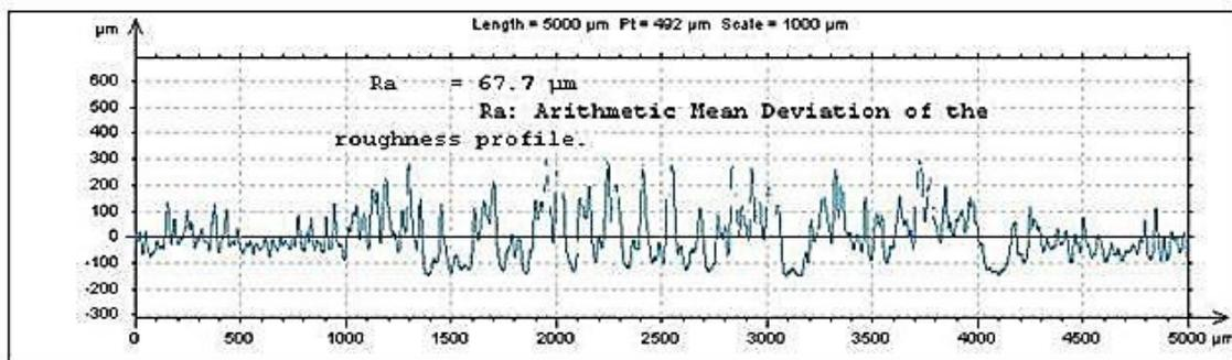
Figure 15. Surface roughness  $R_a$  for test conducted at 450°C
