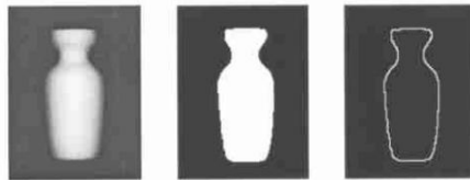
(a)original image; (b) threshold segmentation image; (c) extractive outline
