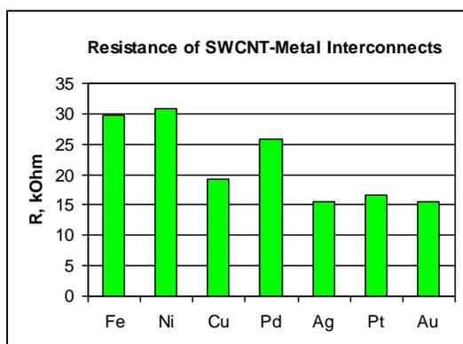
FIGURE 8 Resistances of zig-zag SWCNT-Metal interconnects in comparison.
