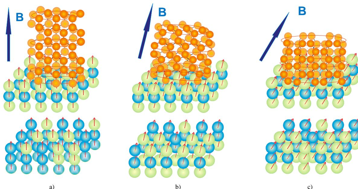
FIGURE 12 Magnetically stimulated orientation of magnetic moments of atoms in model interconnects during the CNTs controlled growth with the expected chiralities under the directed mag  $\phi = \Theta_B$ : a) arm-chair CNT, netic field  $\mathbf{B}$  with the orientation angle  $\Theta_B$ , where  $\mathbf{B}$  is the magnetic induction and the chirality angle is  $\phi = 0^\circ$ ; b) chiral CNT,  $0^\circ < \phi < 30^\circ$ ; c) zig-zag CNT,  $\phi = 30^\circ$
