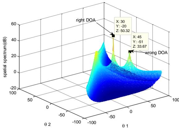
FIGURE 2 Two-dimensional spatial spectrum  $p_c(\theta_1, \theta_2)$  in the case of complex-valued signals for Figure 1,  $\theta_1 = 30^\circ$  and  $\theta_2 = -20^\circ$
