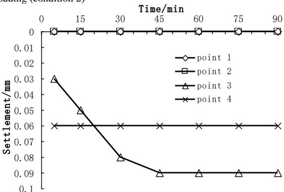
FIGURE 15 Variation of settlement at each point with time at 3.5kPa loading (condition 2)
