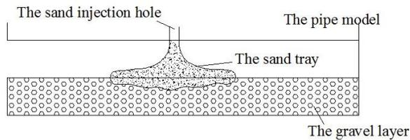
FIGURE 28 Interaction mechanism between sand and gravel
