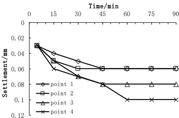
FIGURE 20 Variation of settlement at each point with time at 1.5kPa loading (condition 4)
