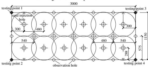
FIGURE 4 Demonstration of the location of injecting holes and observation holes (unit: mm)
