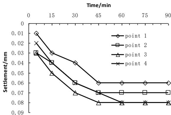
FIGURE 9 Variation of settlement at each point with time at 2kPa loading (condition 1)
