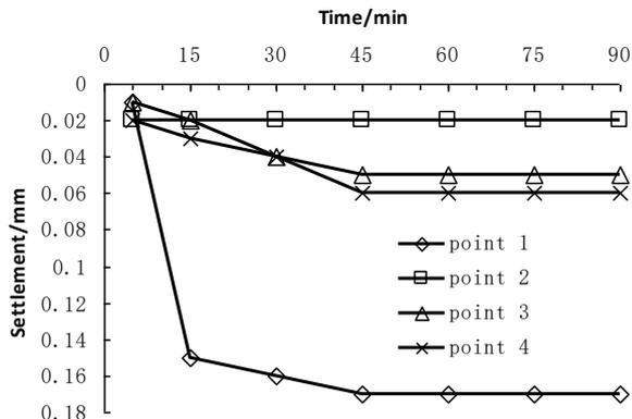
FIGURE 8 Variation of settlement at each point with time at 1.5kPa loading (condition 1)
