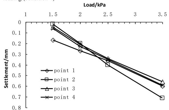
FIGURE 24 Variation of settlement with loading in condition 1
