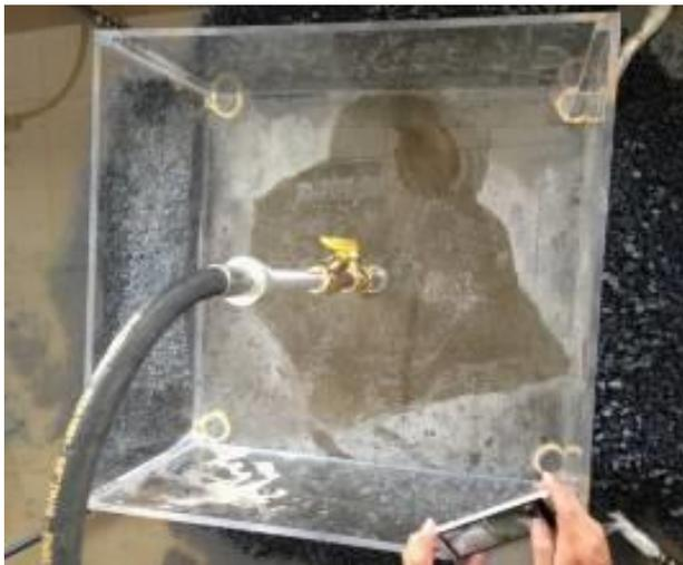
FIGURE 2 Individual sand tray tests
