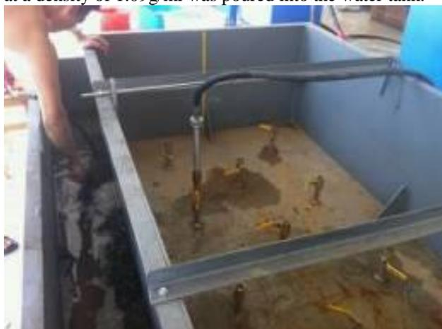
FIGURE 5 Sand injection process
