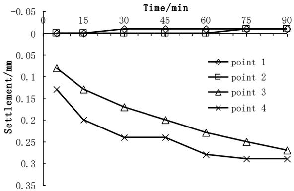
FIGURE 12 Variation of settlement at each point with time at 1.5kPa loading (condition 2)
