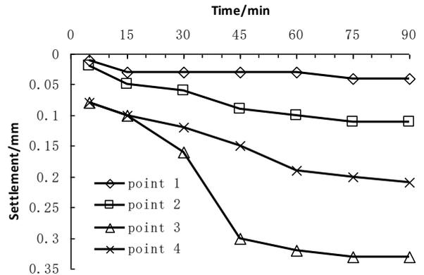
FIGURE 16 Variation of settlement at each point with time at 1.5kPa loading (condition 3)
