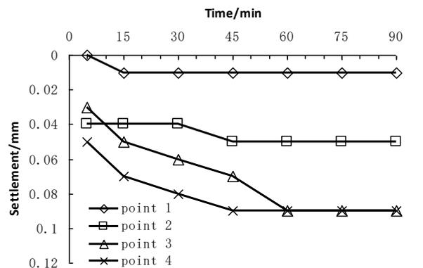
FIGURE 18 Variation of settlement at each point with time at 2.5kPa loading (condition 3)
