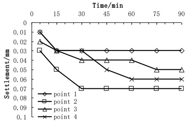
FIGURE 23 Variation of settlement at each point with time at 3.5kPa loading (condition 4)
