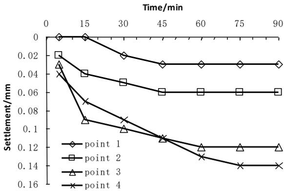
FIGURE 19 Variation of settlement at each point with time at 3.5kPa loading (condition 3)
