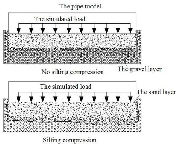
FIGURE 29 Silting influence schematic
