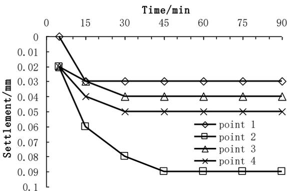
FIGURE 21 Variation of settlement at each point with time at 2kPa loading (condition 4)
