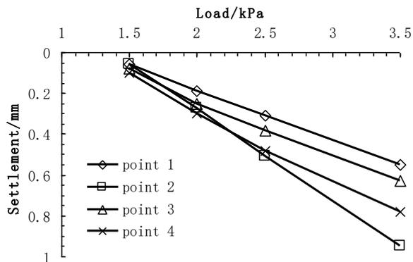
FIGURE 27 Variation of settlement with loading in condition 4
