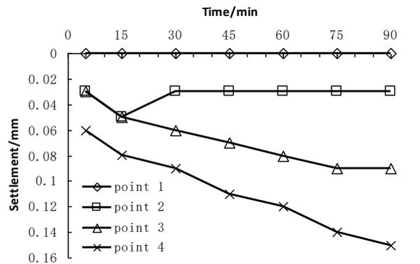
FIGURE 17 Variation of settlement at each point with time at 2kPa loading (condition 3)
