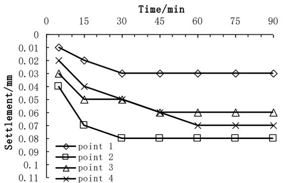
FIGURE 22 Variation of settlement at each point with time at 2.5kPa loading (condition 4)
