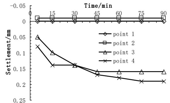
FIGURE 13 Variation of settlement at each point with time at 2kPa loading (condition 2)
