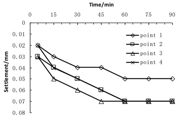
FIGURE 11 Variation of settlement at each point with time at 3.5kPa loading (condition 1)
