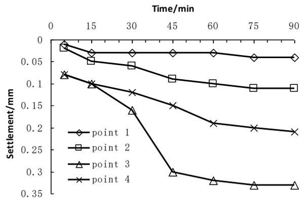
FIGURE 15 Variation of settlement at each point with time at 1.5kPa loading (condition 3)
