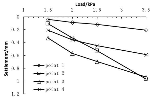
FIGURE 26 Variation of settlement with loading in condition 3
