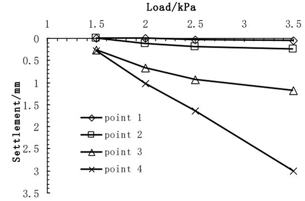
FIGURE 25 Variation of settlement with loading in condition 2
