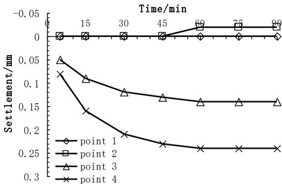
FIGURE 14 Variation of settlement at each point with time at 2.5kPa loading (condition 2)
