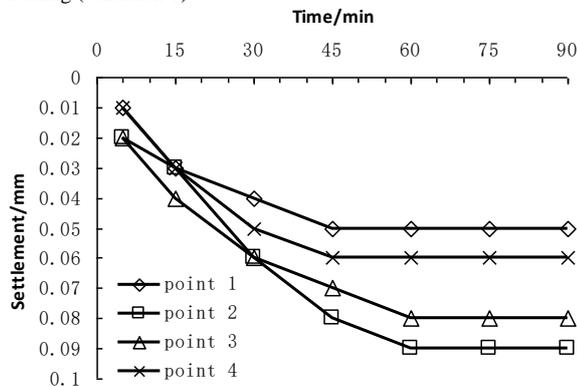
FIGURE 10 Variation of settlement at each point with time at 2.5kPa loading (condition 1)
