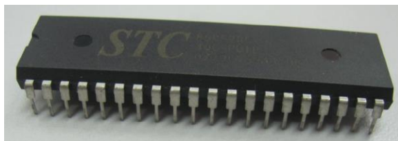
FIGURE 3 The outside view of the MCU
