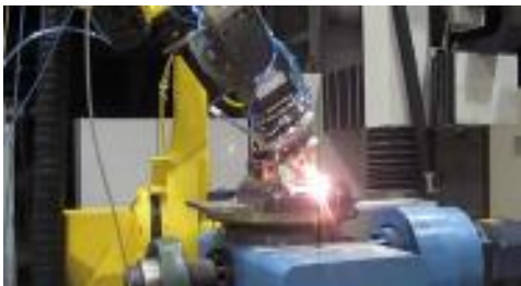
FIGURE 2 Repairing by laser cladding technique
