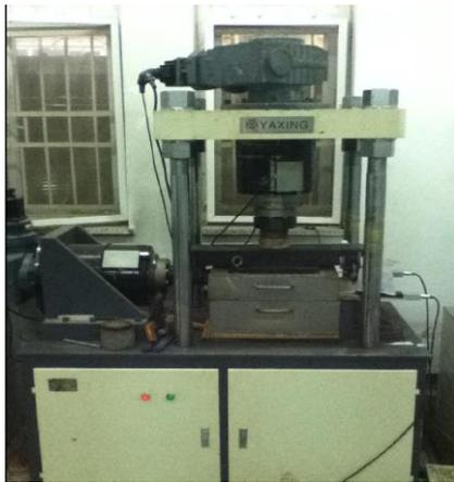
FIGURE 1 Shear test box
