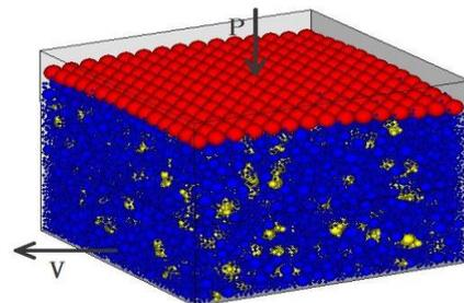
FIGURE 4 DEM model of sub-ballast direct shear test
