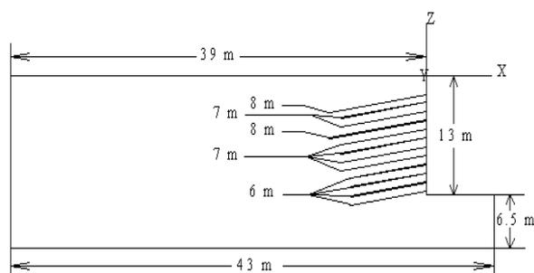
FIGURE 2 The profile of foundation pit support design
