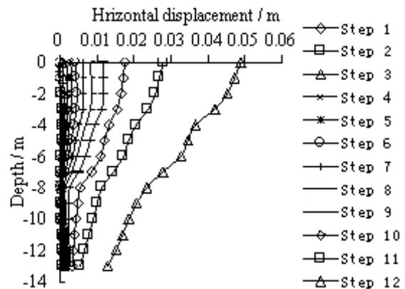
FIGURE 7 The change curve of horizontal displacement with the depth of the excavation that the position away from the excavation surface was 9 m
