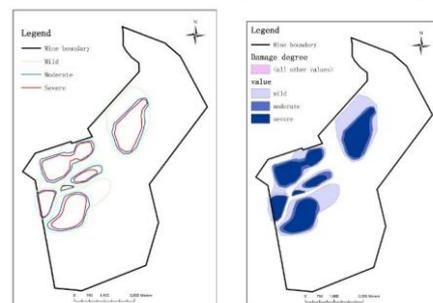
FIGURE 3 Demarcation of land damage based on predicted vertical displacement
