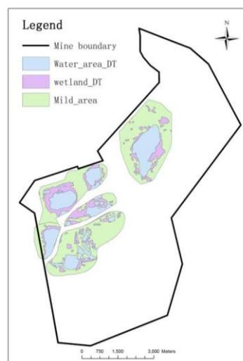
FIGURE 7 Land management map based on vertical displacement predictions and Landsat-8 extraction
