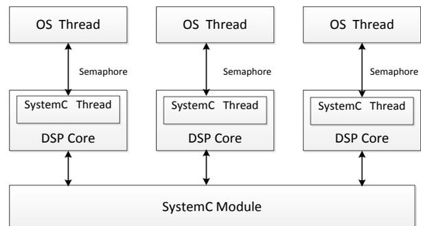
FIGURE 5 SystemC thread parallel optimization
