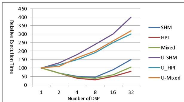
FIGURE 8 Relative execution time of quick sort
