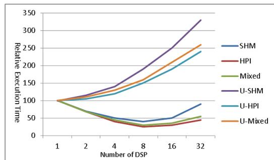
FIGURE 7 Relative execution time of matrix multiplication
