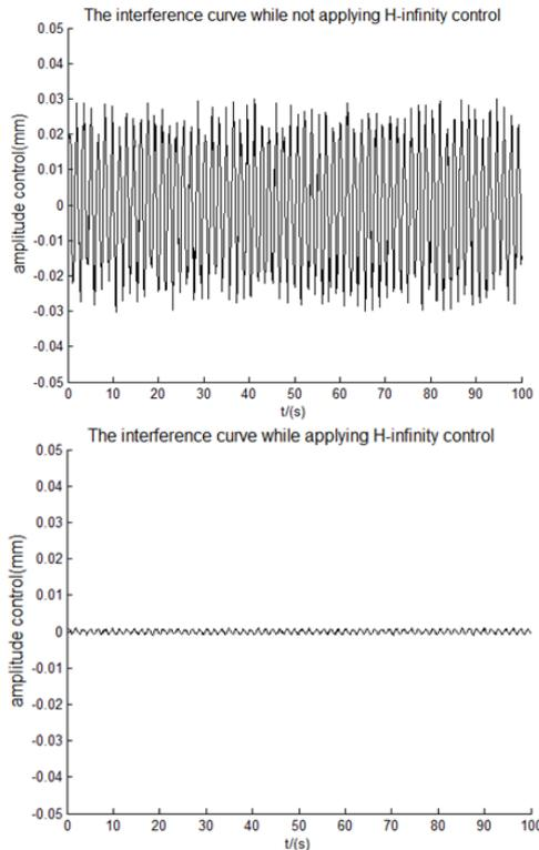
FIGURE 11 Response curves of the wrist joint for disturbance
