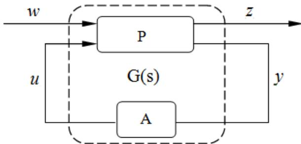
FIGURE1 The general H-Infinity tracking control method for picking- arm
