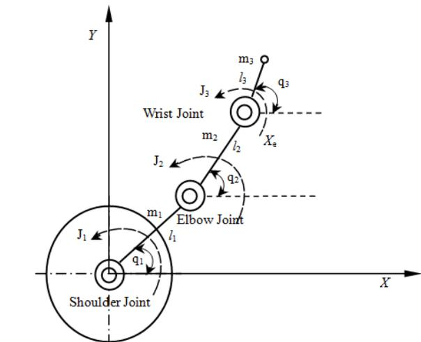
FIGURE 5 The model schematic diagram of picking-arm
