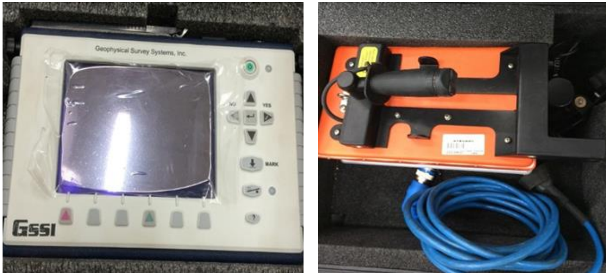
FIGURE 2 Field data manager and the radar antenna
