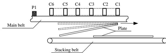
FIGURE 5 dropping control schematic diagram of 1# stacking table magnetic system
