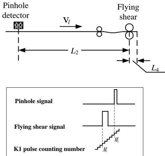
FIGURE 2 Schematic plot of calculating distance  $L_3$
