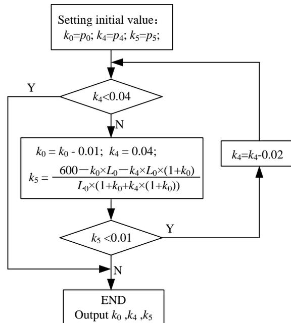
FIGURE 4 speed scale factor calculating algorithm flow
