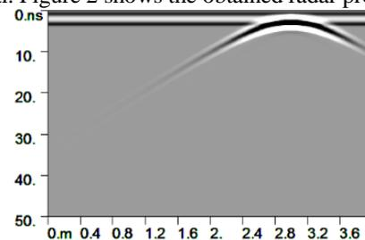
a) Simulated effects of radar profile when survey line parallel to the short axis of collapse column in horizontal
