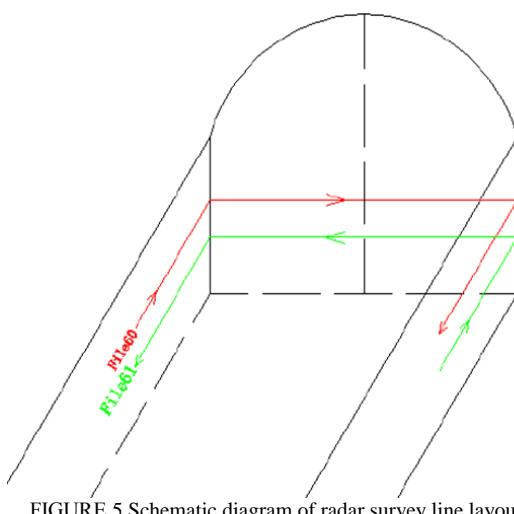
FIGURE 5 Schematic diagram of radar survey line layout
