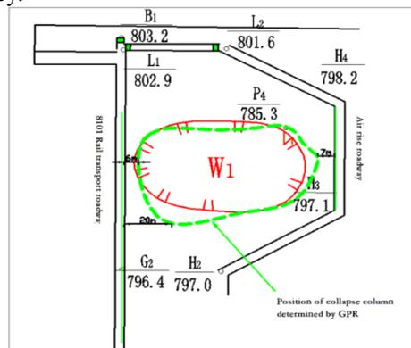
FIGURE 9 Comparison diagram between collapse column positions in radar detection and geological data
