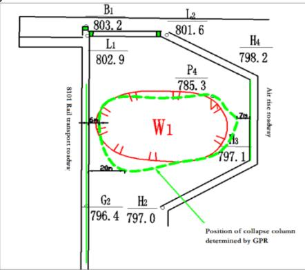
FIGURE 9 Comparison diagram between collapse column positions in radar detection and geological data
