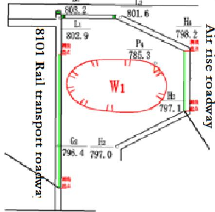
FIGURE 4 Schematic diagram for survey lines of 8101 rail haulage roadway
