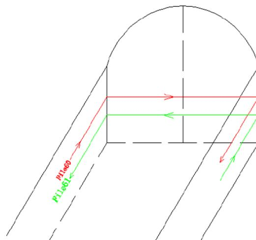
FIGURE 5 Schematic diagram of radar survey line layout
