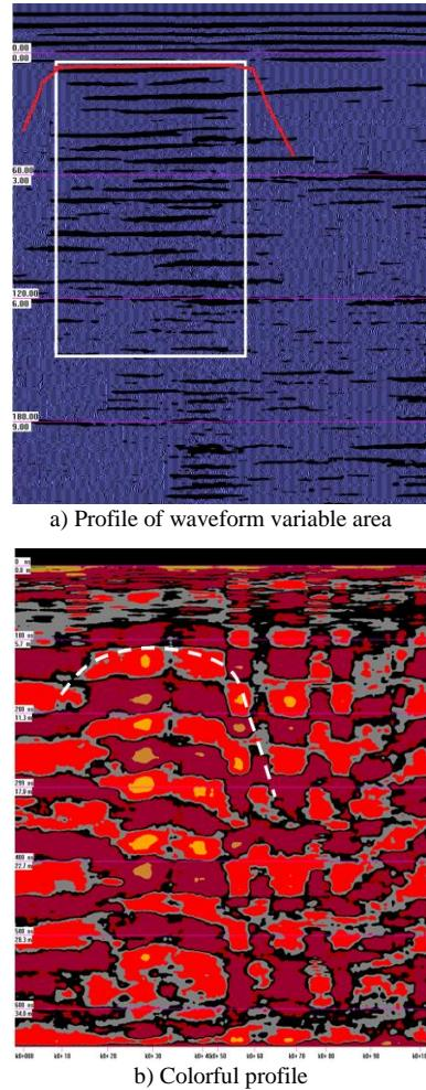
FIGURE 6 Radar detection profile of collapse column in rail haulage roadway
