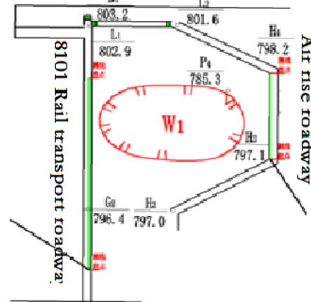
FIGURE 4 Schematic diagram for survey lines of 8101 rail haulage roadway
