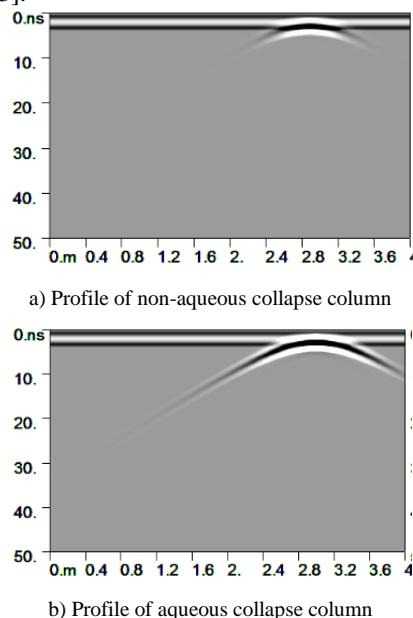
FIGURE 3 Comparison chart for simulated profiles of collapse column with different aqueous conditions
