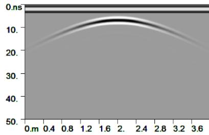
b) Simulated effects of radar profile when survey line parallel to the long axis of collapse column in horizontal
