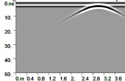
a) Simulated effects of radar profile when survey line parallel to the short axis of collapse column in horizontal
