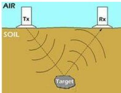
FIGURE 1 Schematic diagram for the principle of ground penetrating radar (GPR) detection
