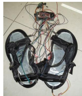
FIGURE4 The position of sensors in insole
