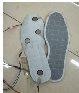
FIGURE3 The package of sensors in the shoes
