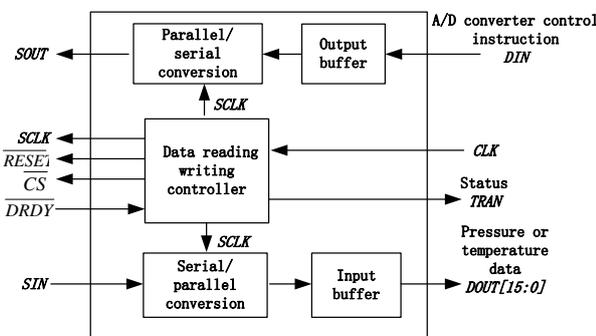
FIGURE 4 Inside block diagram of data reading and writing module
