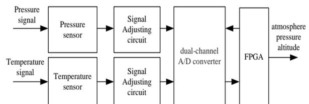
FIGURE 1 Principle diagram of system circuit
