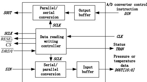
FIGURE 4 Inside block diagram of data reading and writing module
