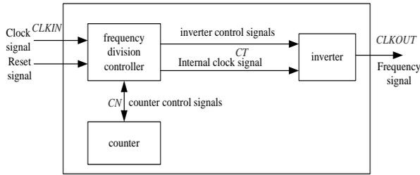
FIGURE 3 Inside block diagram of the frequency dividing module
