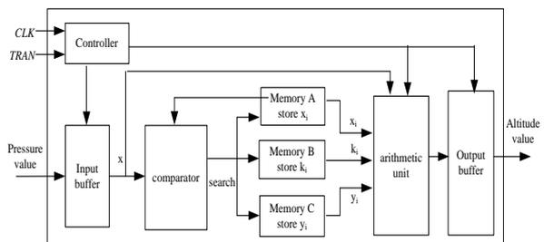
FIGURE 6 Inside block diagram of altitude calculating module
