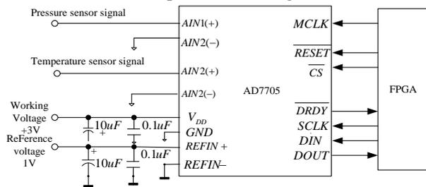
FIGURE 2 Connection diagram of AD7705
