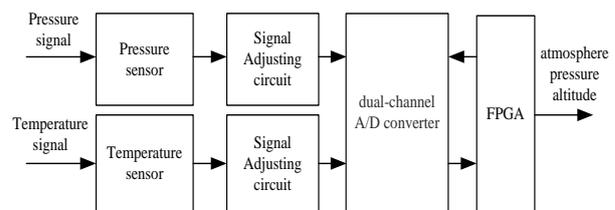
FIGURE 1 Principle diagram of system circuit
