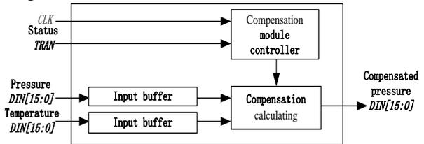
FIGURE 5 Inside block diagram of compensation calculating module
