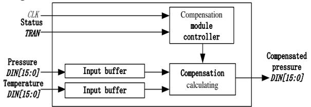
FIGURE 5 Inside block diagram of compensation calculating module
