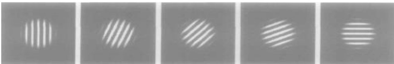
FIGURE 2 Changes in texture direction of 2D Gabor filter function with the real part of the parameter \varphi_\mu
