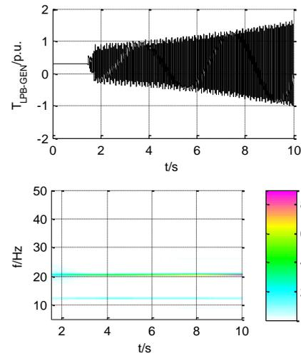
FIGURE 4 The torque response curve between LPB and GEN and its time-frequency contour map (Pe=0.3p.u.)
