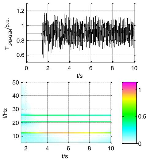
FIGURE 1 The torque response curve between LPB and GEN and its time-frequency contour map (XC=30%)
