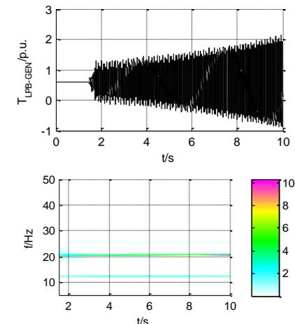
FIGURE 5 The torque response curve between LPB and GEN and its time-frequency contour map (Pe=0.6p.u.)
