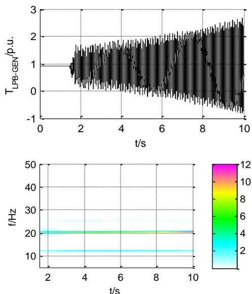
FIGURE 2 The torque response curve between LPB and GEN and its time-frequency contour map (XC=50%)
