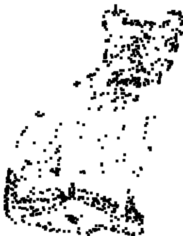
FIGURE 5 Result of making a boundary judgment for each point
