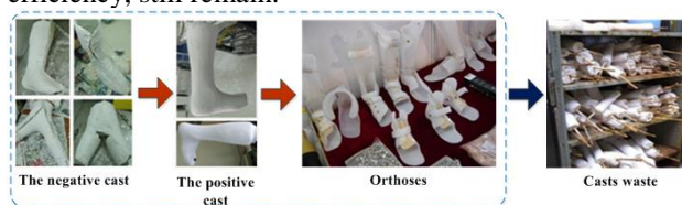
FIGURE 1 Traditional manufacturing of foot orthoses
