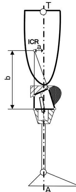
FIGURE 16 The stability parameters of bionic leg.
