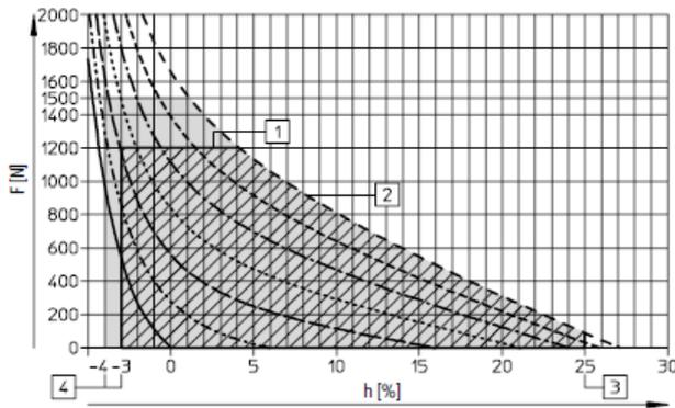
FIGURE 13 The characteristic curves of FESTO-MAS-20-200N-AA-MC-O-ER-EG
