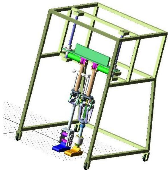
FIGURE 17 Virtual prototype of simplified BRHL
