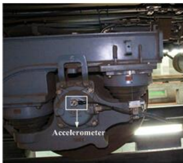
FIGURE 2 Sensor layout of the test vehicle
