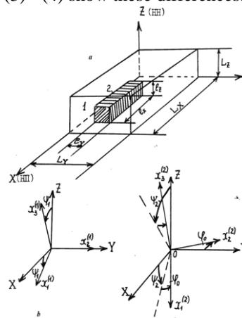
FIGURE 3 Model structure: 1 is an external matrix; 2 is an inclusion, b, c are the principal axes of the conductivity tensor matrix (texture component {110} <112>) and inclusion (texture component {112} <111>),  $\psi_1=30^\circ$ ,  $\psi_2=35^\circ$ ,  $\varphi_0=39^\circ$ .
