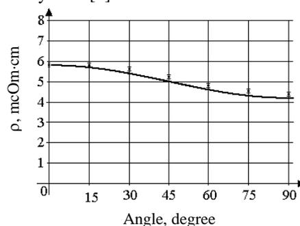
FIGURE 1 Changes of the resistivity of D16 alloys a result of quenching and rolling; the points correspond to experimental results; the solid line is obtained theoretically
