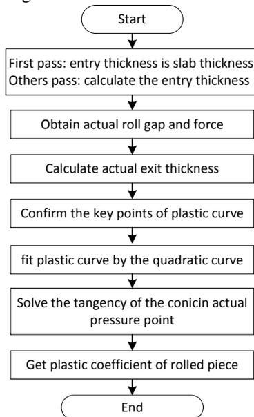
FIGURE 4 Calculation diagram of plastic coefficient
