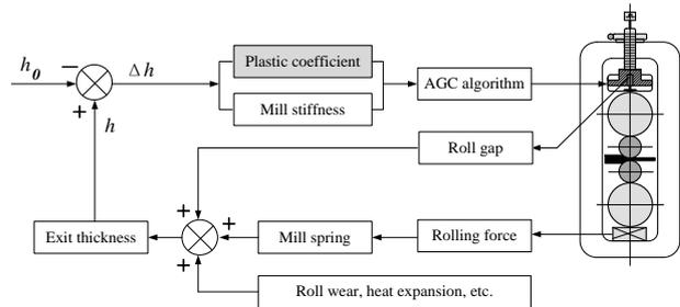
FIGURE 2 Schematic diagram of system for thickness control
