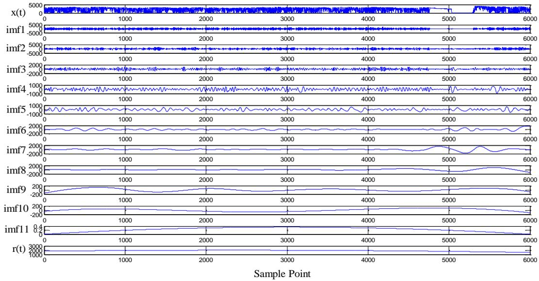
FIGURE 3 Leakage Signal and its IMFs after EMD
