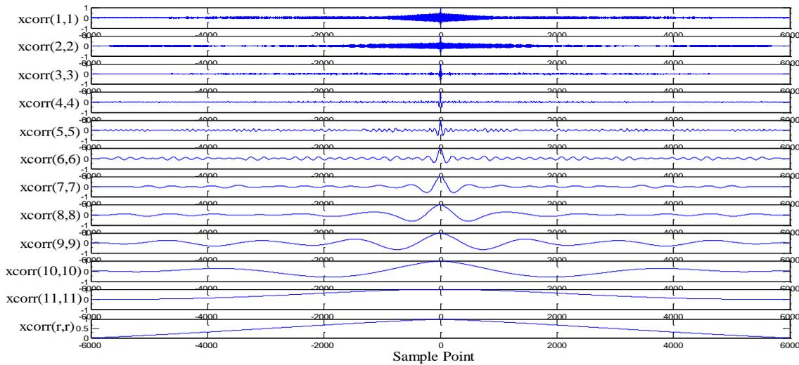
FIGURE 4 Cross-correlation of Leakage Signals and IMFs
