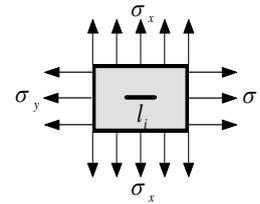
FIGURE 3 The micro crack of representative volume element
