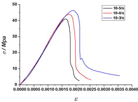
FIGURE 1 The constant strain rate stress-strain curves
