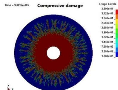
FIGURE 6  $t=90\mu s$  coupled pressure-shear damage moiré pattern
