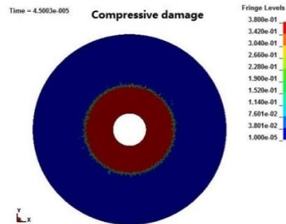
FIGURE 5  $t=45\mu s$  coupled pressure-shear damage moiré pattern
