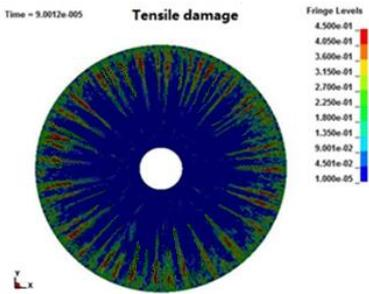
FIGURE 8  $t=90\mu\text{s}$  tensile damage moiré pattern
