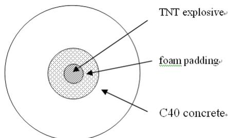
FIGURE 4 The calculation model
