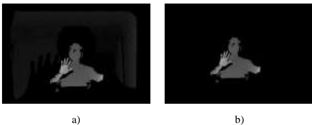
FIGURE 2 a) The original depth image, b) The image after first time thresholding, which had been removed the background
