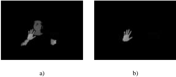
FIGURE 3 a) After applying the threshold to the input image, which is fusion of the depth image and colour image, only the skin colour area is kept. b) After the final phase processing, the detected hand looks like this
