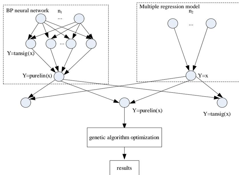
FIGURE 3 Hybrid neural network based on optimized genetic algorithm
