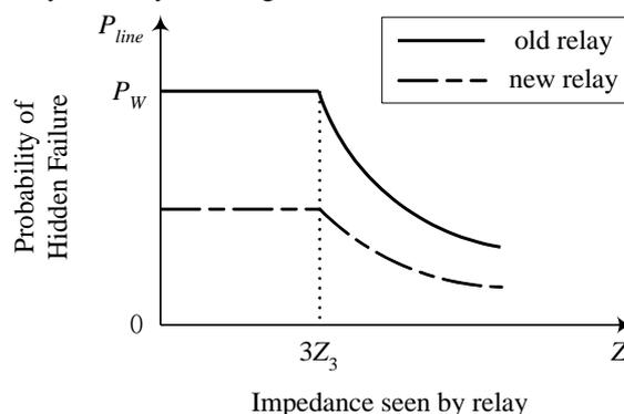
FIGURE1 Hidden failure probability in a line-protective relay
