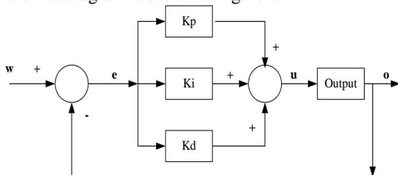
FIGURE 2 Diagram of PID control
