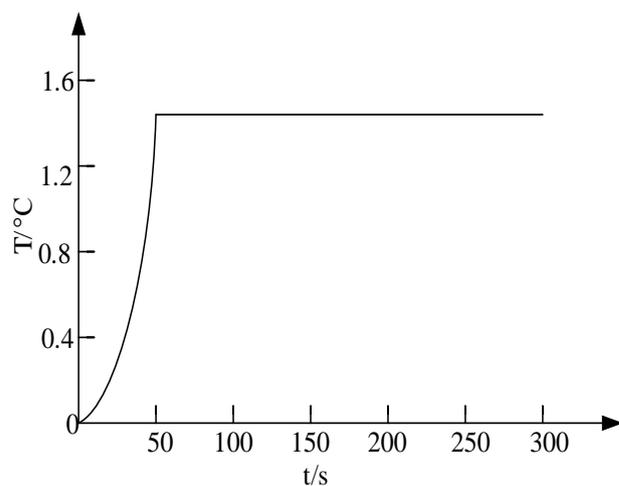
FIGURE 6 Temperature adjustment performance of fuzzy controller
