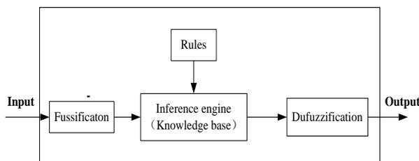
FIGURE 3 Structure of Fussy Block
