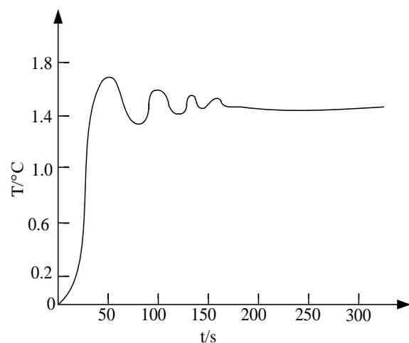
FIGURE 7 Temperature adjustment performance of PID controller
