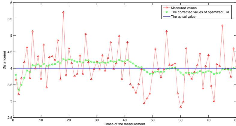
FIGURE 7 Distance data for the first set of measurements
