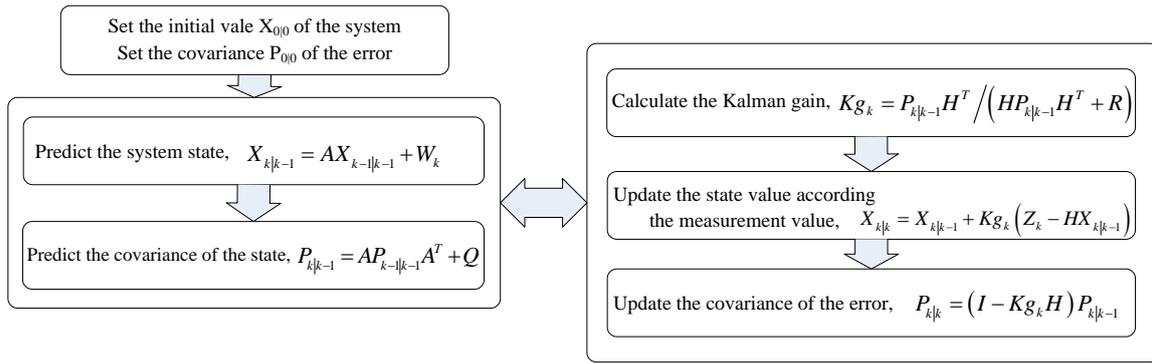
FIGURE 2 Recursive process of the Kalman filter algorithm
