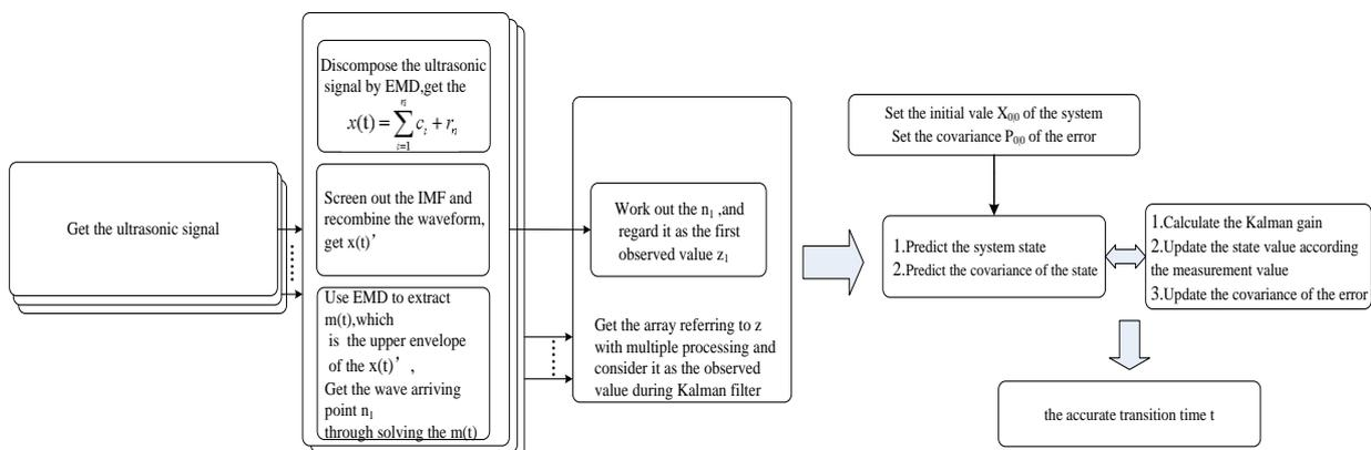
FIGURE 4 Process of the optimized extended Kalman filter algorithm
