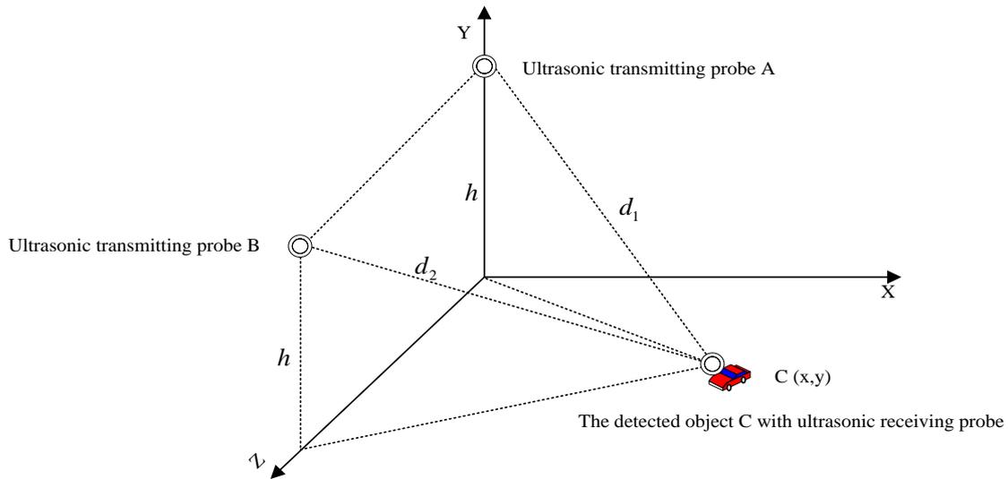
FIGURE 1 Basic structure of the ultrasonic-wave ranging system
