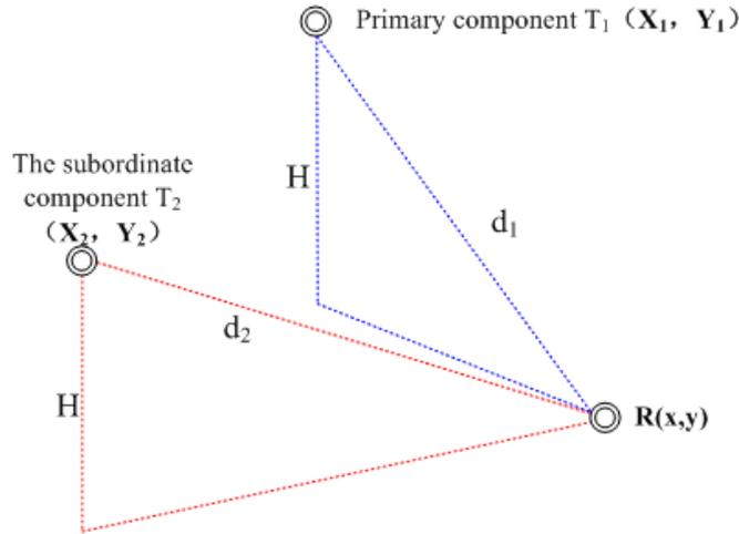
FIGURE 5 Ultrasonic ranging system
