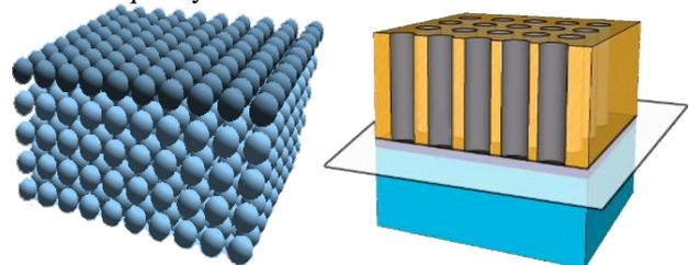
FIGURE 2 The model crystal (on the left) and the model for pulsating ion currents (on the right)
