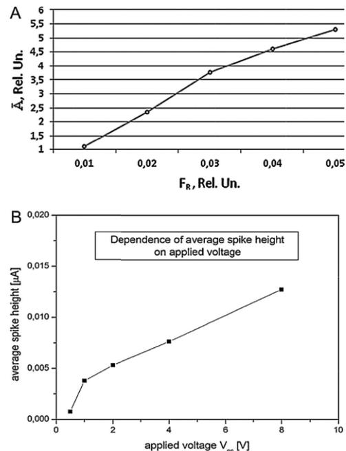
FIGURE 4 Dependence of the average amplitude of MP oscillations on the value of SF (on top); Dependence of the average spike height on the value of the applied voltage (down)
