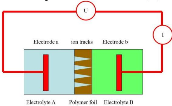
FIGURE 1 Principle arrangement of experimental setup to study current spike emission in ion track-containing foils embedded in electrolytes (current/voltage measurements)
