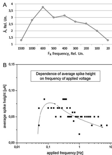
FIGURE 5 Dependence of the average amplitude of MP oscillations on the frequency of SF action (on top); Dependence of the average spike height on the frequency of applied voltage (down), here the curve is drawn by the method of least squares.
