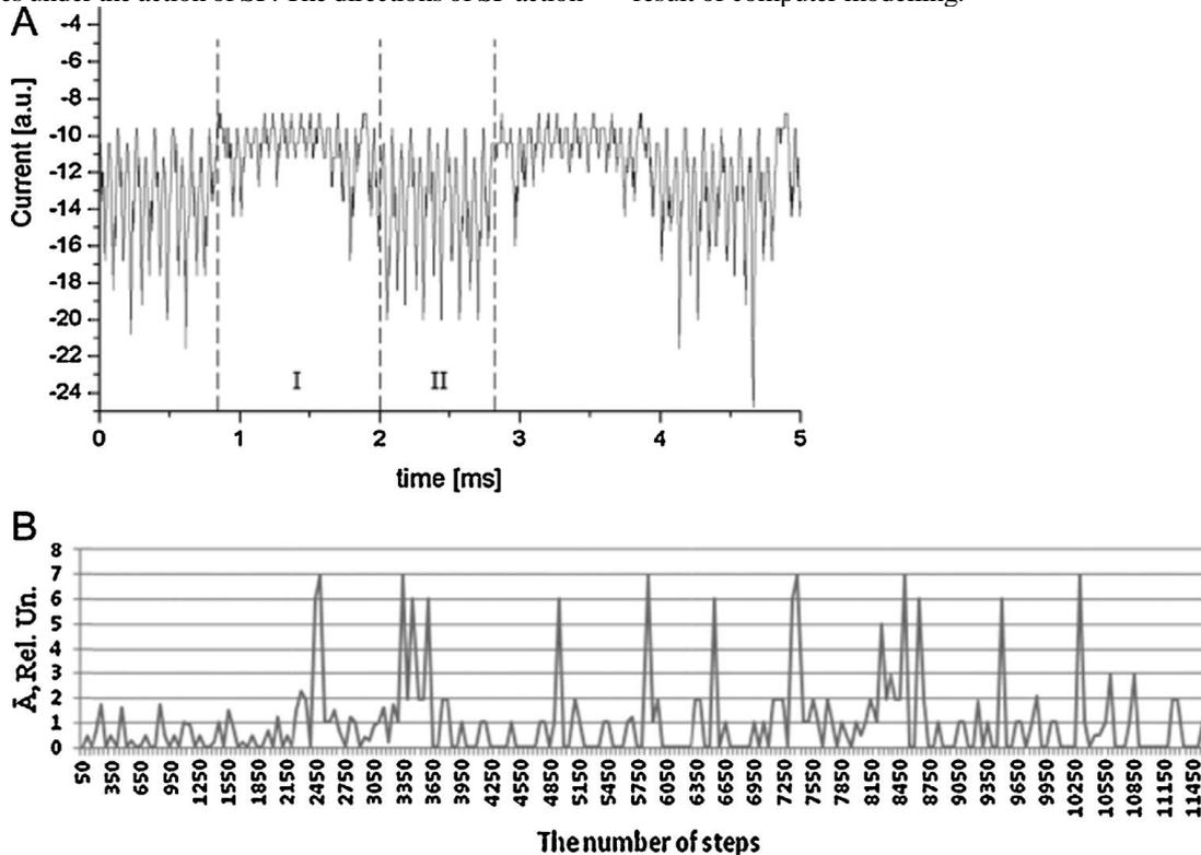
FIGURE 3 Current spikes in conditions of real experiment (on top). Region I corresponds to regular oscillations, region II corresponds to current spikes. Illustration of model spikes in the model experiment (down). At the horizontal axis is the average amplitude of MP oscillations.
