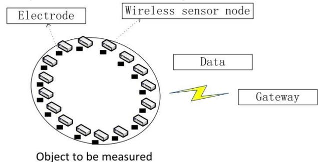
FIGURE 2 model for wireless distributed data acquisition system
