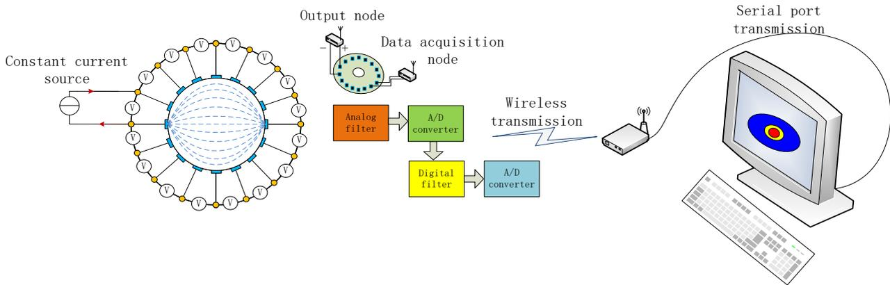
Dimension of the wireless distributed node was 28mm×21mm×13mm. Its small size provided more possibility to be set as close to the electrode as possible. In most cases, the wire between node and electrode was not longer than 15 mm, which might cause amount of noise interference.
