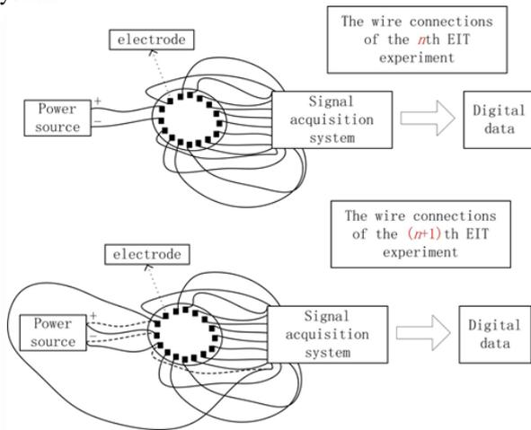
FIGURE 1 the wire connections of the parallel systems
