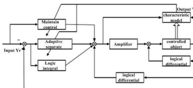
FIGURE 1 Adaptive control structure based on characteristic model
