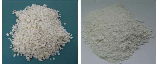
FIGURE 3 before and after the cushion test of quartz sand
