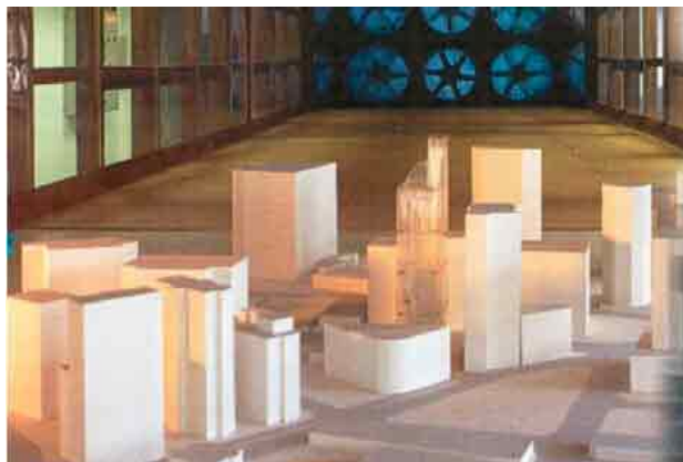
FIGURE 2 Building model in a wind tunnel
