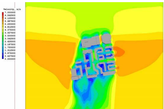
FIGURE 15 Wind velocity distribution of plan one of modern trade mart in winter at the height of 1.5m
