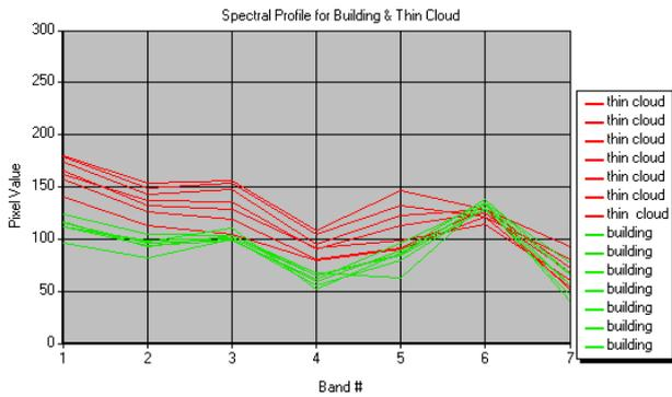
FIGURE 5 The spectral profile of building and thin cloud
