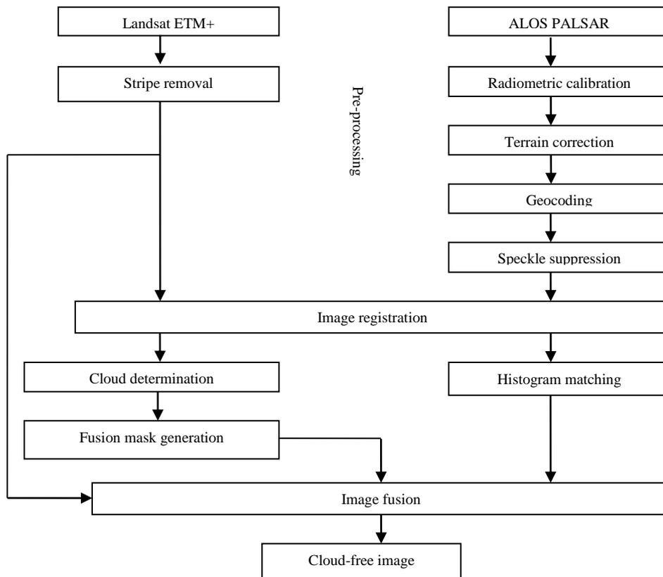
FIGURE 3 The whole processing framework of cloud removal
