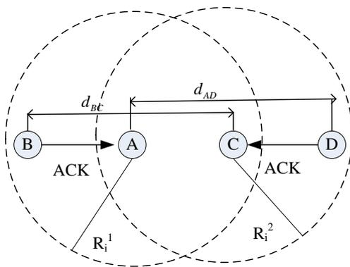
FIGURE 3 Transmitting ACK Frame when Concurrent Transmission
