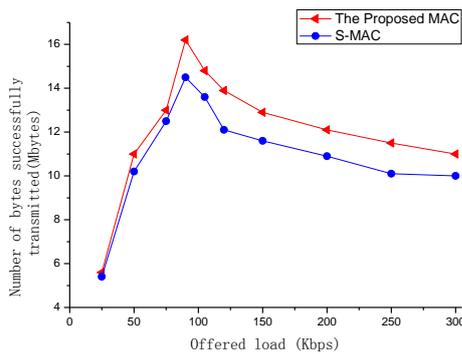
FIGURE 6 Throughput versus with offered load
