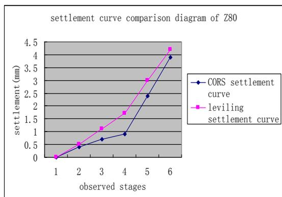
FIGURE 4 Settlement curve comparison diagram of Z80
