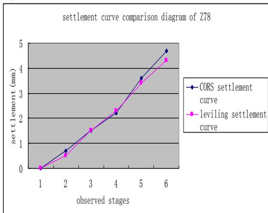
FIGURE 2 Settlement curve comparison diagram of Z78
