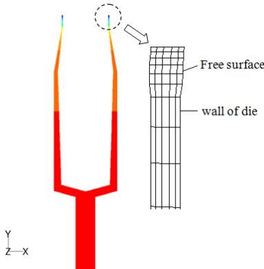
FIGURE 5 The shape of free surface in extrusion segment using the grid replacement method
