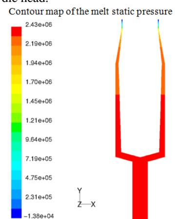
FIGURE 4 contour map of the melt static pressure
