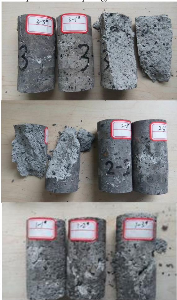
FIGURE 3 Different proportion specimen compression broken pattern
