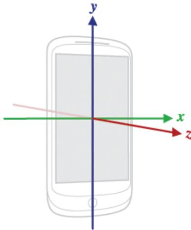
FIGURE 1 The coordinate system of the Android Smart Phone
