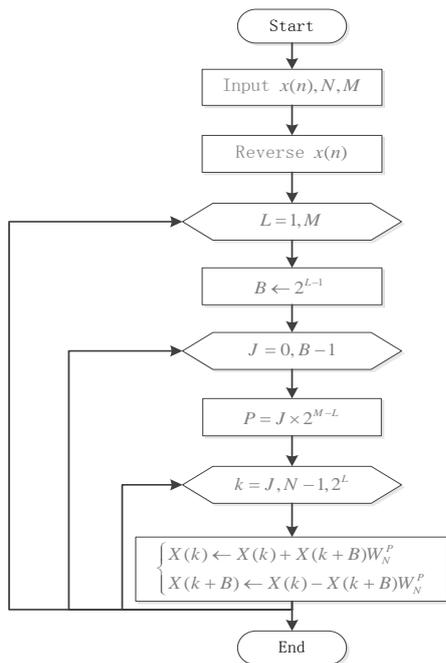
FIGURE 3 The flow chart of the FFT algorithm
