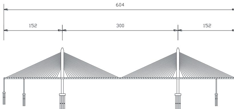
FIGURE 8 The elevation of Fanhe bridge (unit: m)
