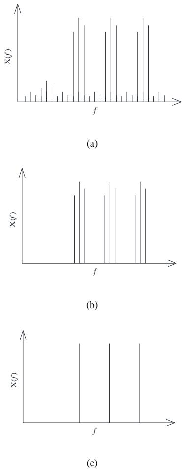
FIGURE 4 The steps of determining the natural frequencies
