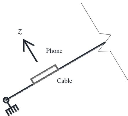
FIGURE 2 The fixation of a mobile phone on the cable
