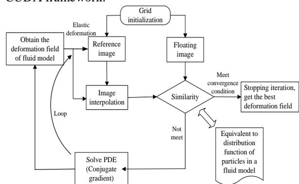
FIGURE 5 Improved viscous fluid registration algorithm of medical images
