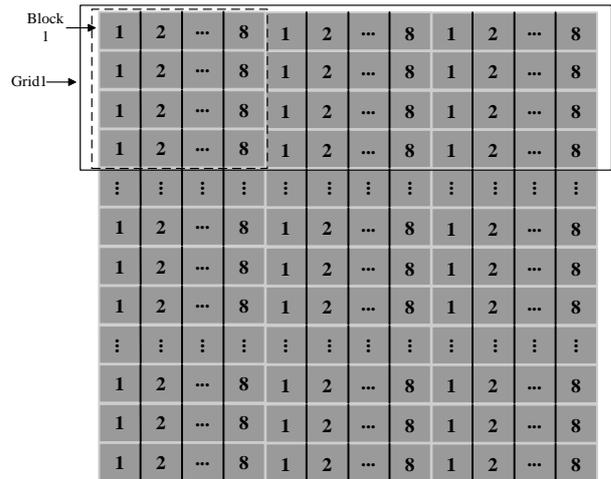
FIGURE 3 Division of the block and grid in Fluidproc()
