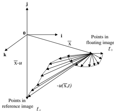
FIGURE 1 Description of the displacement field of the Eulerian reference frame
