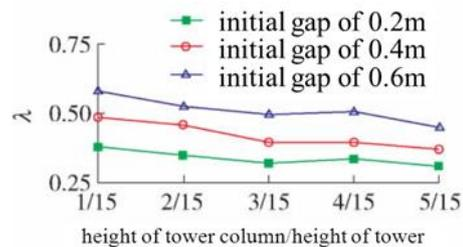
FIGURE 9 Relative displacement variation at left expansion joint resulted from collision
