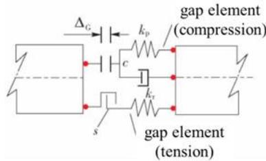
FIGURE 2 Model of expansion joint
