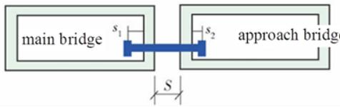
FIGURE 1 Coupling beam device
