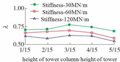
FIGURE 17 Variation of relative displacement on the left side induced by collision
