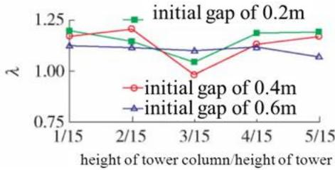
FIGURE 11 Variation of bending moment of fixed pier of left approach bridge caused by collision
