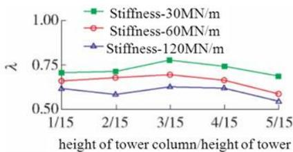
FIGURE 18 Variation of relative displacement on the right side induced by collision
