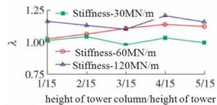
FIGURE 15 Variation of bending moment of the fixed pier bottom of the left approach bridge caused by collision
