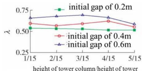
FIGURE 10 Relative displacement variation at right expansion joint induced by collision
