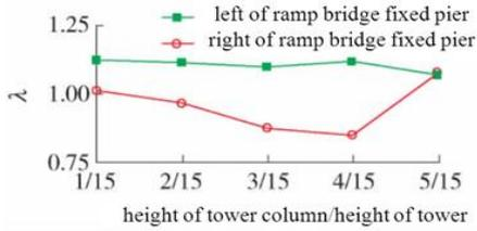
FIGURE 5 Variation of shear force on key section of the bridge
