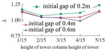
FIGURE 12 Variation of bending moment of fixed pier of right approach bridge caused by collision
