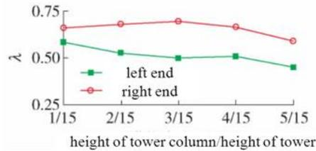
FIGURE 6 Variation of relative displacement at expansion joint
